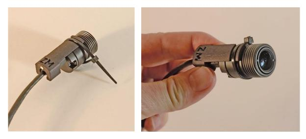
Place it over the camera/connector. Use a cable tie to secure the assembly.
