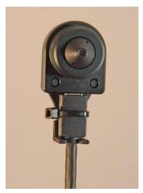
Place the strain it over the camera/connector. Use a cable tie, if needed.
