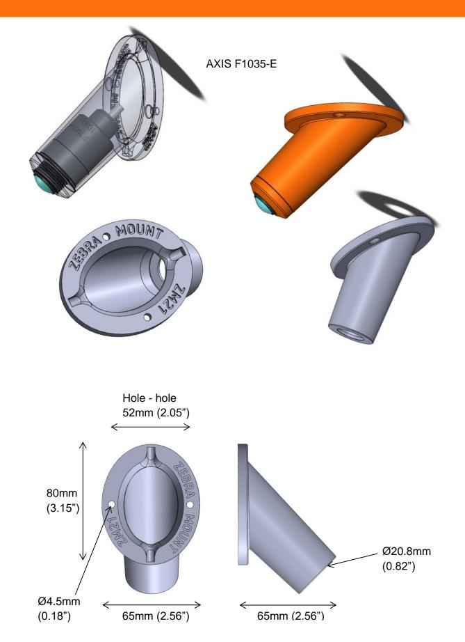
The design is made for countersunk screws.
