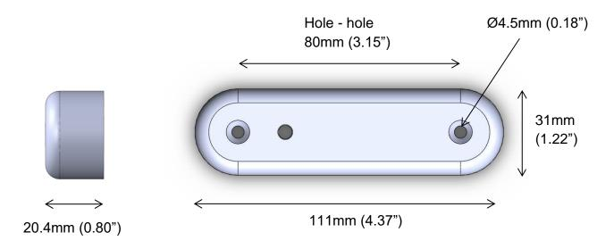
The design is made for countersunk screws.
