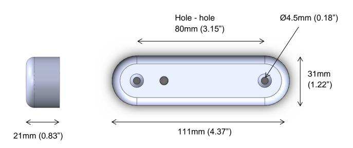
The design is made for countersunk screws.
