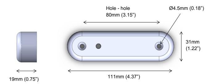
The design is made for countersunk screws.
