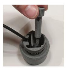
Separate the three parts, using a wire cutter, before mounting the camera. Mount the camera at a steep angle before placing the lens in its hole.
