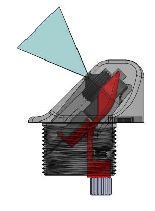
Attach the camera to the sledge. Place the sledge into the casing. Secure the sledge with the screw. Mount the casing using a 1-1/4" locknut.
