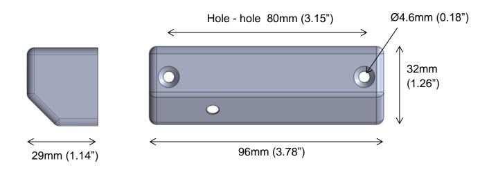
The design is made for countersunk screws.
