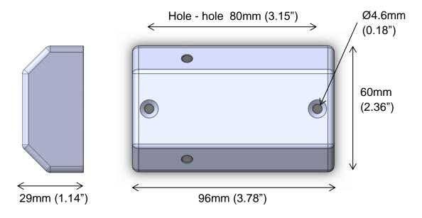
The design is made for countersunk screws.
