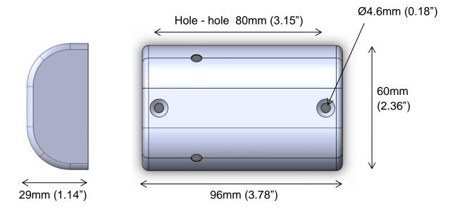
The design is made for countersunk screws.
