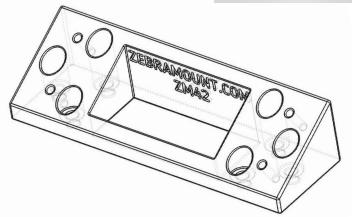
Four screws are needed to attach the door station mounting plate to the wedge. E.g. 4.2x13mm or #8x1/2" screws will work.
